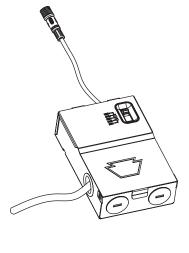
Insert driver box into ceiling in accordance with local/ national codes and connect the male and female connectors. Screw threaded nut over connectors to secure.
