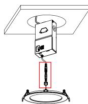
**8.** Lifting both retention tabs upward, push the fixture into the hole until trim sits flush with ceiling.
