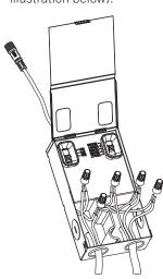
**6.** Place all wiring and connections back into the box and close the cover.
