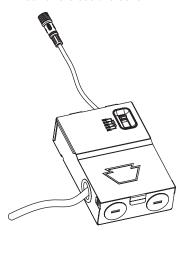
7. Insert driver box into ceiling in accordance with local/ national codes and connect the male and female connectors. Screw threaded nut over connectors to secure.
