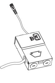
7. Insert driver box into ceiling in accordance with local/ national codes and connect the male and female connectors. Screw threaded nut over connectors to secure.
