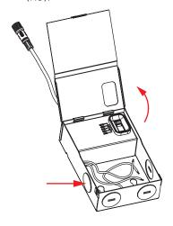
**5.** Insert the electrical supply cable through the KO; use appropriate bushing to prevent wire abrasion. Wire driver box (see Wiring Diagram on page 3 and illustration below).\*
