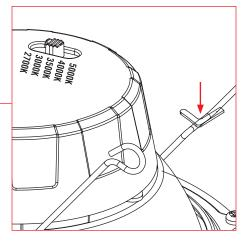
**8.** Carefully route wires into fixture and push recessed kit up flush to ceiling surface.
