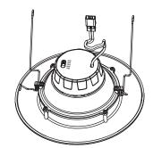
**6.** Plug E26 base cable connection into the recessed housing, ensuring that kit is grounded .
