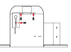
**3.** Remove existing socket mounting plate from the housing, then remove lamp socket from the plate.
