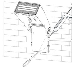
6. Adjust luminaire to the desired position
