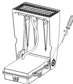
3. Open holes for corresponding junction box screws. If predefined template does not match with junction box, drill additional holes
