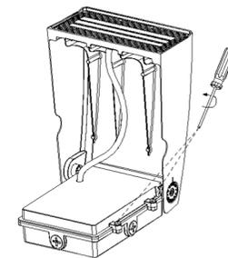
3. Open holes for corresponding junction box screws. If predefined template does not match with junction box, drill additional holes
