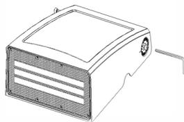
2. Open the back housing, disconnect the quick connector (between LED module and LED driver) inside the fixture and remove the front housing
