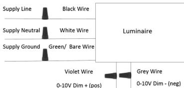
This high-quality product has been designed for use with a low voltage 0-10V dimmer. **DO NOT USE WITH STANDARD WALL DIMMER**
