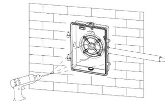
5. Connect LED quick disconnect, close the luminaire and apply silicon around the luminaire perimeter.
