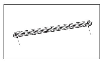
8. Secure lens to housing with lens latches.
