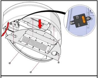
**Step 1:** With the supply power off, open the bottom cover and carefully detach the LED reflector assembly. Adjust the controller to the desired wattage by sliding the switch on the controller.
