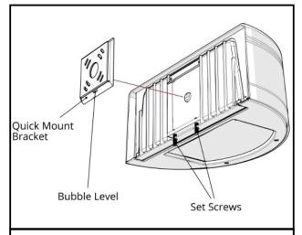
**Step 2:** Remove the quick mount bracket from the fixture and attach it to the junction box with the appropriate hardware (not included).
