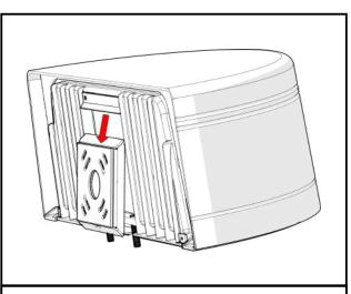
**Step 4:** Lift the fixture and tilt slightly toward the quick mount bracket. Hook the fixture housing onto the quick mount bracket as shown. Take care not to pinch any wires.
