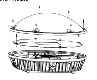
Reroute wires coming out of ¾" hole and seal the hole with provided plug. Drill 4 holes on four corners and fix it onto the ceiling with suitable screws.
