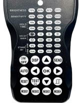
**Daylight Sensor Setting:** Sensor setting to only allow the luminaire to illuminate below a defined ambient brightness threshold. Daylight sensor is active only when luminaire is off. (default disabled; fixture turns on whenever motion is detected)
