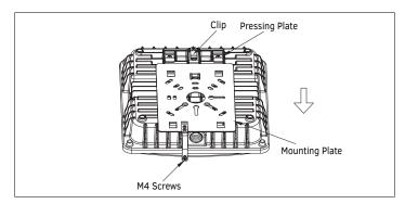
3. Connect the clip of the fixture to the spindle of the mounting plate to ensure the fixture will not slip and fall. Complete wiring using the wiring diagram, then push the pressing plate into the suspension loop on the mounting plate.
