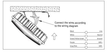
Attach the mounting plate to the ceiling using M16 Expansion Bolts or M6 stainless steel screws with plastic anchors (not included).
