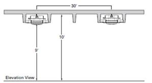
NOTE: 1 Vertical reading is taken at lowest point of horizontal illumination level.
