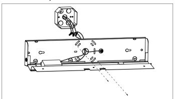
6. Reattach the lens onto the luminaire housing.
