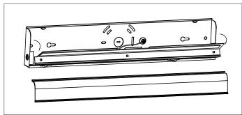
2.Remove the lens and LED driver cover from the luminaire.
