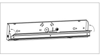
2.Remove the lens and LED driver cover from the luminaire.
