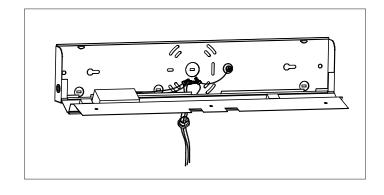
6. Reattach the lens onto the luminaire housing.
