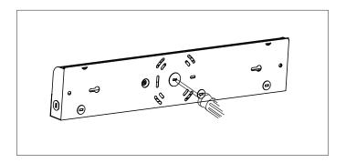
3.Position the luminaire housing in the desired location,and then mark and drill mouting holes at the narrow ends of the keyhole slots. Screw in mounting screws leaving space for channel body. Slide channel over mounting screws. Lift and shift channel into position and tighten screws.
