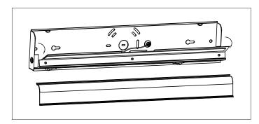
4.Make connections from the incoming power wires to the driver input power wires.Position the junction box mounting holes over the junction box and secure.
