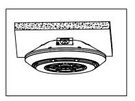
Like picture A, Unscrew the plug, adjust wattage and cct as desired, and tighten the plug.
