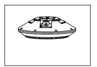
2.Connect the wires threaded from conduit and canopy,Black wire for Line,White for Neutral,Yellow Green for ground
