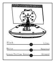
4.Slide the Canopy lights into bracket, and secure the screw on side of the light to prevent the light sliding out from the bracket. Installation done.
