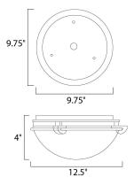
MEASUREMENTS DIMENSION : 12.5" L x 12.5" W x 4" H HANGING WEIGHT : 2.82 lb LAMPING INPUT VOLTAGE :120V : 2 x 60W Incandescent E26 Medium , 120W Total BULB **BULB INCLUDED** : (Not Included) DIMMABLE
