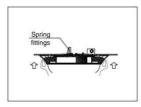
3. Install the assembled lamps to the ceiling. Use shrapnel to position the lamp on the ceiling and lock the fixtures.
