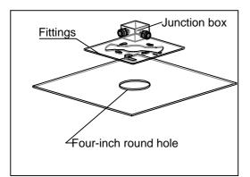
1. Place the installation board on the ceiling (the ceiling is metal) and keep the four-inch round hole concentric.
