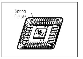
2. Put the shrapnel on the LED light, then tighten the shrapnel with two screws.
