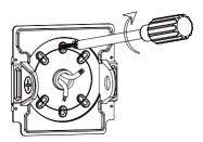
7. Fix the fixture by 4 screws
