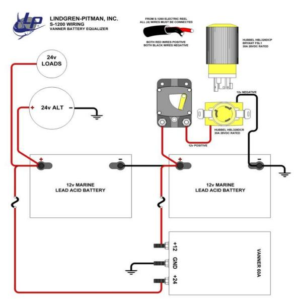
Minimum Wire Sizes from Battery to Outlet: 0 to 10 feet - 8 AWG 10 to 20 feet - 6 AWG For runs greater than 20 feet please call customer service to discuss your options.
