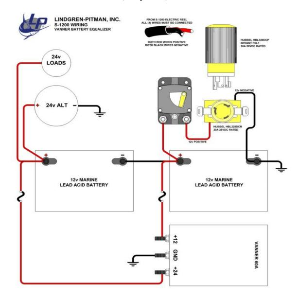
$\begin{array}{c} \mbox{Minimum Wire Sizes from Battery to Outlet:} \\ \mbox{0 to 10 feet - 8 AWG} \\ \mbox{10 to 20 feet - 6 AWG} \end{array}$
