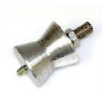
The hour glass rollers are key to holding the monofilament aligned for proper line setter performance. They do not require any maintenance, but if bearings do fail the complete hour glass roller must be replaced.
