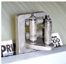
2 – level winder shaft bearings ( do not over grease )
