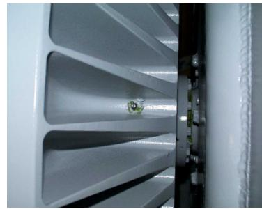
( Zerk mounted on spool between end ribs ).
