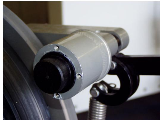
The contact wheels will outlast the drive elements many times. Severe wear can effect line setter performance and when a deep groove is worn from the monofilament the rubber drive element cannot perform properly and the upper idler contact wheel must be replaced.
