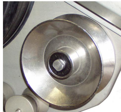
The V - groove pulley does not require replacement from wear of the pulley. When bearings are worn they should be replaced. No special tools or procedure is required. The v-groove pulley is mounted from a 1/2" - 13 N.C. threaded stud formed on the axle end. It also has "wrench flats" to facilitate proper tightening and removal.
