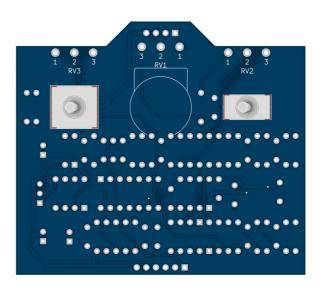
65: Locate the 3 potentiometers and remove all mounting hardware. Grip the small metal tab on each pot with a pair of pliers and gently rock the tab until it snaps off.
