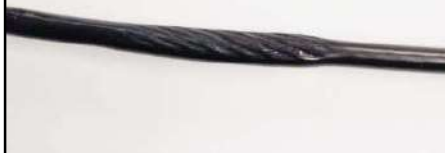
STRETCHED, FRAYED OR FLATTENED CABLE COVERING
