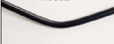
A BREAK OR PERMANENTLY BEND IN THE CABLE
