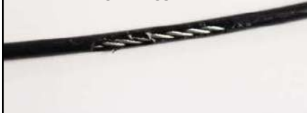
A TEAR, TWISTING/BINDING IN THE CABLE COVER
