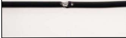
FRACTURES IN THE CABLE COVER
