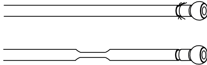
STRETCHED, FRAYED OR FLATTENED CABLE COVERING
