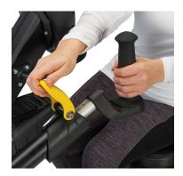
Pull up on lever to unlock.
