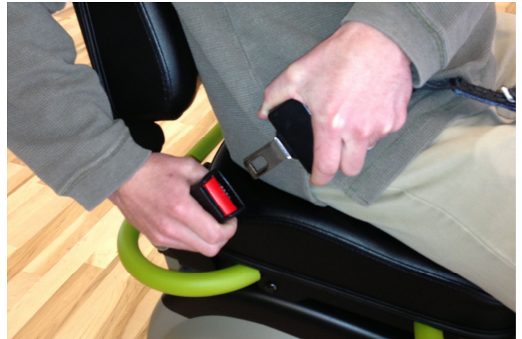
Retractor being clipped into Buckle
