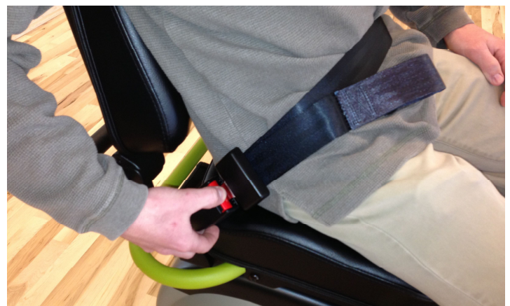
Red Button on Buckle being pressed to Release Belt
