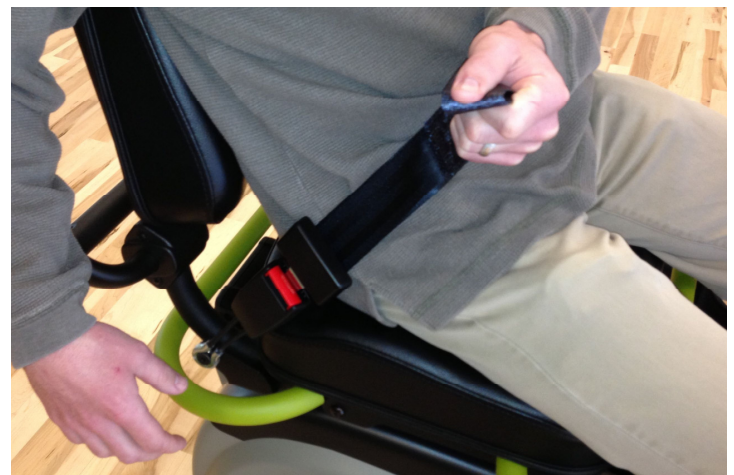
Adjuster loop being pulled to take up slack
