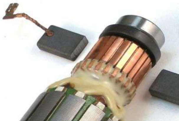
After: Brushes look like stainless steel surface and armature bright gold.
