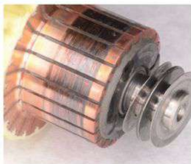
Before: Needs cleaning & resurfacing with cleaning stone
