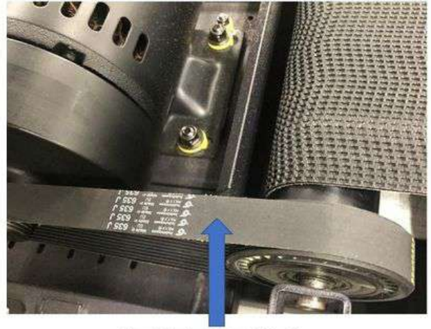
Adjust drive belt to 125HZ to 135HZ with Frequency Gauge or Smart Phone Guitar APP.
