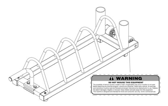
The Warning Label shown here has been placed on the Rack Storage Frame. If the label is missing or illegible, please call customer service at 1-800-999-8899 for replacement. Apply the label in location shown.
