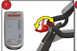
Move the shift lever from stop to stop 6 times.
