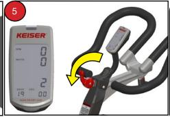
Set shift lever to gear 19 for Miles, or set shift lever to gear 21 for Kilometers.
