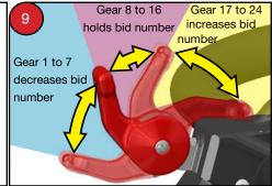
Once the trip units have been set, you have the opportunity to adjust the bike id number. Adjust the shift lever to attain the desired bike id number. Set the shift lever to any number between gear 8 and 16.
