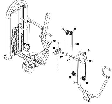
Insert one end of the weight belt (28) through the slot in the top plate belt clamp until approximately one inch of the free end of the belt protrudes from the slot in the opposite side of the clamp.
