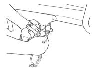
Screw the coupling cap to the threaded Y cable housing end.
