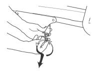
8. Align arrows then insert the pendant cable end into the Y cable housing.
