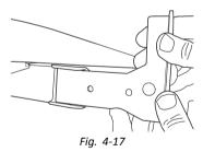
6. 76 inch Bed Only - Slide the bed end bracket in the mounting channel. Align the hole in the bracket with the channel hole.
