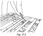
7. Cut the untrimmed or green tie holding the mattress keepers on either side of the bed.
