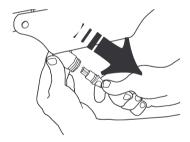
On the other side of the bed, remove the cap from the Y cable housing. Replace the cap on the other side of the bed.
