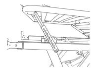
5. To reset the ratchet mechanism, raise the platform to the highest level then lower the platform in one motion.
