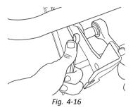
5. 76 inch Bed Only - Remove the fasteners on the bed end bracket.
