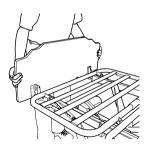
5. Guide the key through the small bracket hole. The key is attached to the bed bracket with a lanyard.
