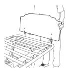
3. Slide the boards down while plate/post screws are in the bracket slots.
