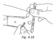
8. 76 inch Bed Only - Tighten the fasteners with two 7/16 inch wrenches. Reposition the other three brackets and reapply the ends.
