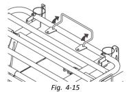
4. 76 inch Bed Only - With a 7/16 inch socket wrench and 7/16 inch wrench loosen and remove the bed end bracket fasteners.
