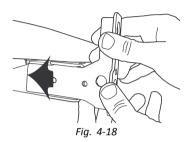
7. 76 inch Bed Only - Reinsert the bed end bracket fasteners.
