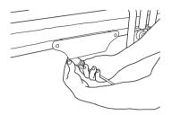
6. Remove the cable end from the Y cable housing.
