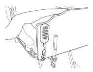
5. To move the pendant to the other side of the bed, disconnect the main power then unscrew the coupling cap on the pendant cable.
