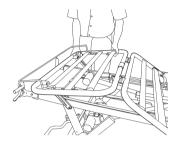
2. The foot section can rest at any of the six pre-set stops.
