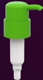
162HX2J28410S281 Specification: \Phi 28/410 (E= 25.5 T=28 H=14.5) Dosage/Output: 2.3 \pm 0.3ml/T
