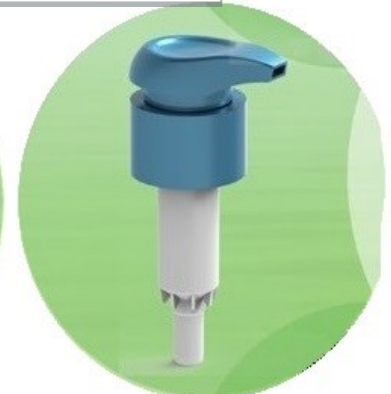
162N20L24410S241 Specification: \Phi 24/410 (E= 22.1 T=24.3 H=14.1) Dosage/Output: 2.3/2.8 \pm 0.2ml/T ZL201530486245.5
