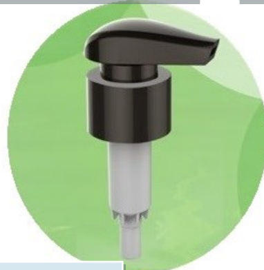
162N20Y28410S281 Specification: \Phi 28/410 (E= 25.5 T=28.0 H=14.5) Dosage/Output: 2.3/2.8 \pm 0.2ml/T ZL201730132030.2
