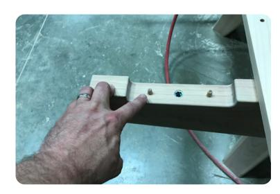
**12** Install 8mm dowel pins to the long base frame.
