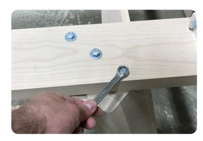
**10** Fix loosely crossmembers to legs using 3/8"-16 x 2 1/2"hexagonal bolts ans 7/16" flat washers.
