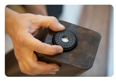
Unwrap legs and unscrew leg levellers for about 1/2".
