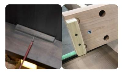
**16** Attach the frame to the playing surface and cross members with wood screws #8 x 1 1/4" round headed Also use the large holes underneath the net crossmember to fix the surface.
