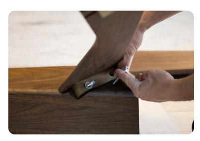
On one table leg, fix one of the short spacers using 1/4"-20 x 2" machine screws and 5/16" washers. These same screws/washers will be used until step 9.
