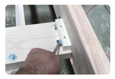
Tighten all bolts and machine screws.
