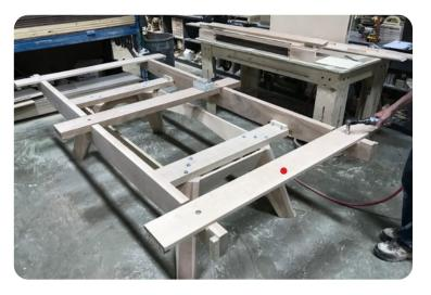
Fix crossmembers to base framesusing 3/8"-16 1 1/4" hexagonal bolts and 13/32" flat washers and the net crossmember with 3/8"-16 1 3/4" hexagonal bolts and 13/32" flat washers. HOLE ON DRAWER SIDE.
