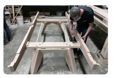
**11** Fix loosely both long base frames to the legs using 3/8"-16 x 1 3/4" hexagonal bolts and 7/16" flat washers.
