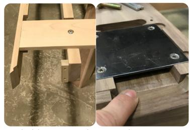
**9** Fix both long aprons to the crossmembers using 1/4"-20 x 1 1/2" machines screws and 5/16" flat washers. TO FACILITATE THE INSTALLATION OF THE CHROME POLES (OPERATION 13) BE SURE THAT THE POINTED SURFACES ARE LEVELED.
