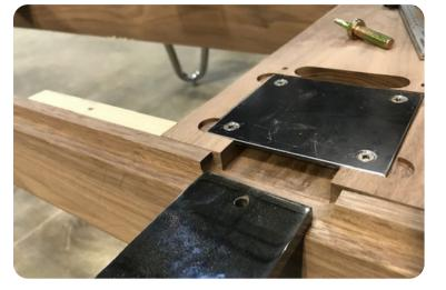
**13** Slide both chrome poles in place into the net crossmember underneath the metal plate.
