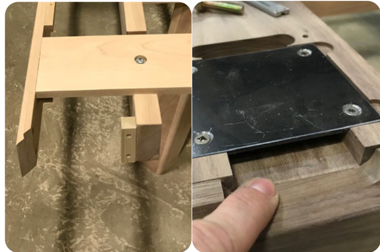
9 Fix both long aprons to the crossmembers using 1/4"-20 x 1 1/2" machines screws and 5/16" flat washers. TO FACILITATE THE INSTALLATION OF THE CHROME POLES (OPERATION 13) BE SURE THAT THE POINTED SURFACES ARE LEVELLED.
