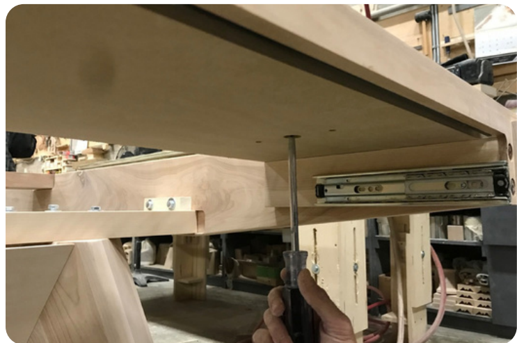
12 Repeat operations 10 and 11 for the second short apron or, for a product with a drawer, fix the drawer's box to the crossmember using 1/4"-20 x 1/2" machine screws and machine screws 1/4"-20 x 1/2" (round head). to the apron.
