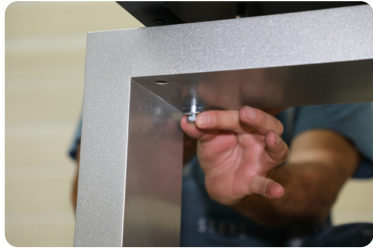
8 While raising one end of the assembled base frame, slide underneath and fix one leg with 3/8"-16 x 3" bolt and 7/16" flat washers. Repeat for other leg.
