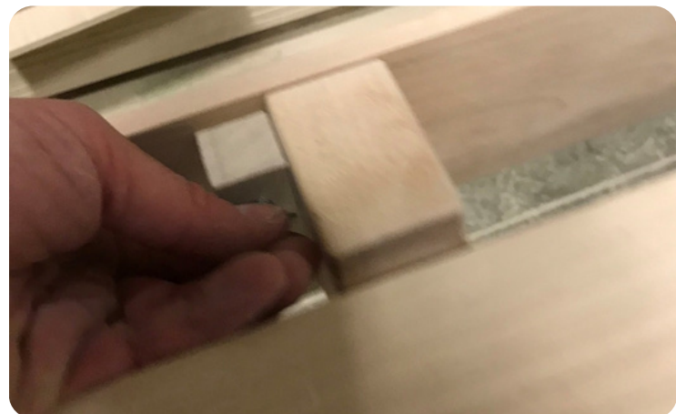
11 Fix this same short apron to the long base frames with 1/4"-20 x 1 1/2" machines screws and 5/16" flat washers
