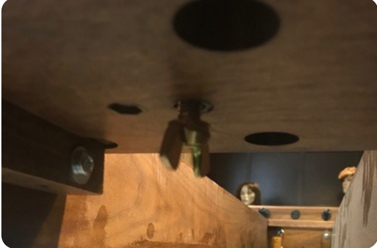
16 Loosely screw the 3/8"-16 x 1 1/2" winged nut underneath the net crossmember. This nut will allow you to tighten the net or completely remove the chrome poles when using your table as a dining table.
