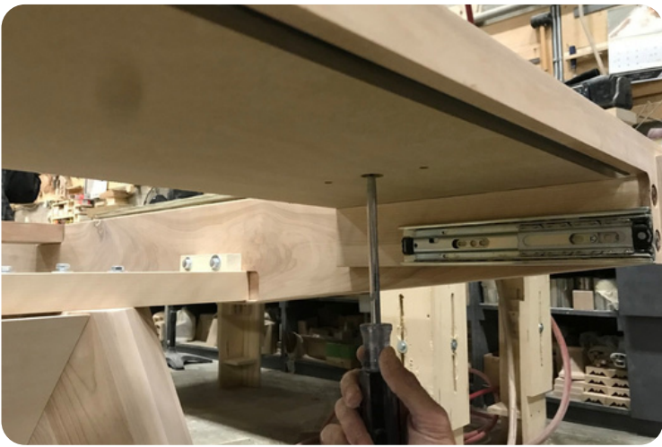
13 Repeat operations 11 and 12 for the second short apron or, for a product with a drawer, fix the drawer's box to the crossmember using 1/4"-20 x 1/2" machine screws and machine screws 1/4"-20 x 1/2" (round head). to the apron.
