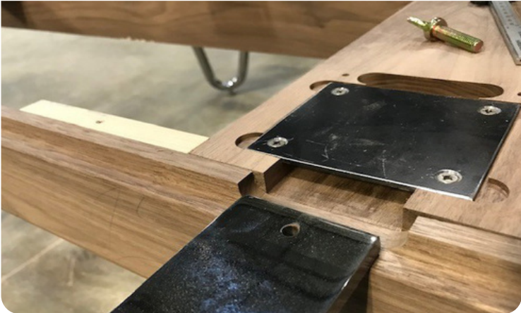
15 Slide both chrome poles in place into the net crossmember underneath the metal plate.
