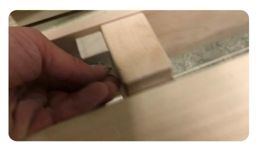
**11** Fix this same short apron to the long base frames with 1/4"-20 x 1 1/2" machines screws and 5/16" flat
