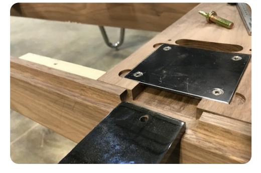
**13** Slide both chrome poles in place into the net crossmember underneath the metal plate.
