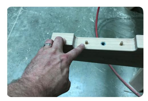
4 Install 8mm dowel pins to the long base frame.
