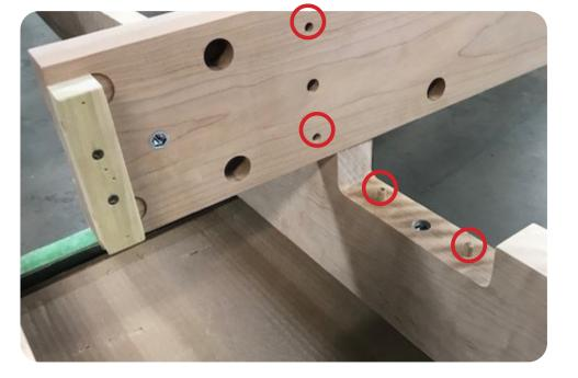
**7** Using the dowel pins for alignement, install the net crossmembers (thicker crossmember).
