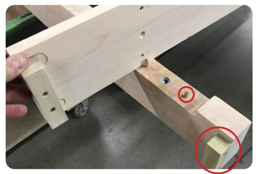
Using the dowel pins for alignement, install the tiner crossmembers. Be sure that the blocs on the long base frames.are oriented on the outside of the a s s embl y.
