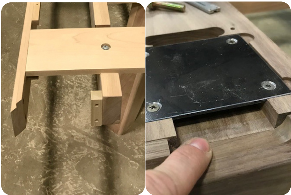
9 Fix both long aprons to the crossmembers using 1/4"-20 x 1 1/2" machines screws and 5/16" flat washers. TO FACILITATE THE INSTALLATION OF THE CHROME POLES (OPERATION 14) BE SURE THAT THE POINTED
