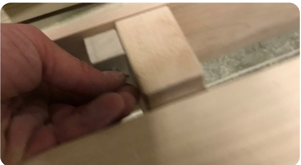
11 Fix this same short apron to the long base frames with 1/4"-20 x 1 1/2" machines screws and 5/16" flat
