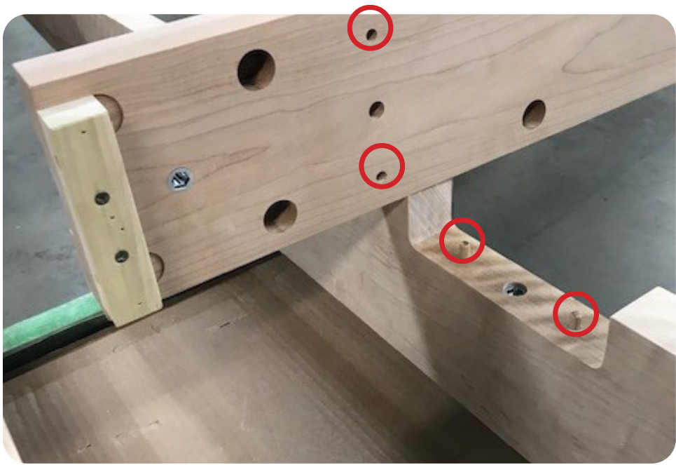
7 Using the dowel pins for alignment, install the net crossmembers (thicker crossmember).
