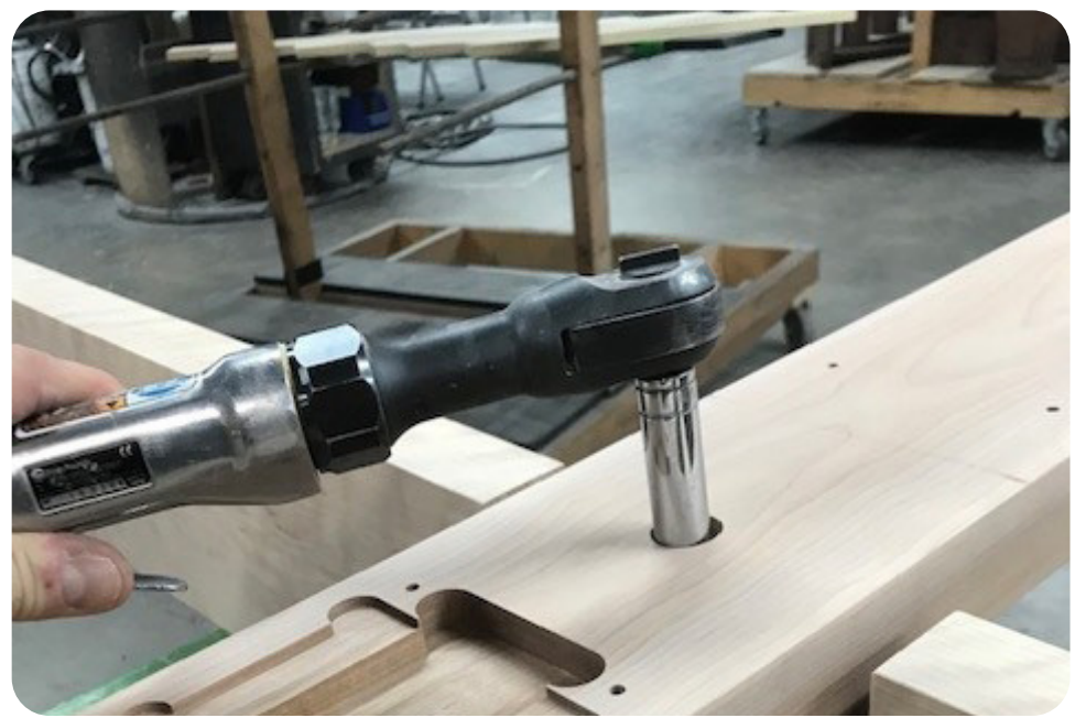
8 Fix the net crossmember with 3/8"-16 x 1 3/4" hexagonal bolts and 13/32" plat washers.
