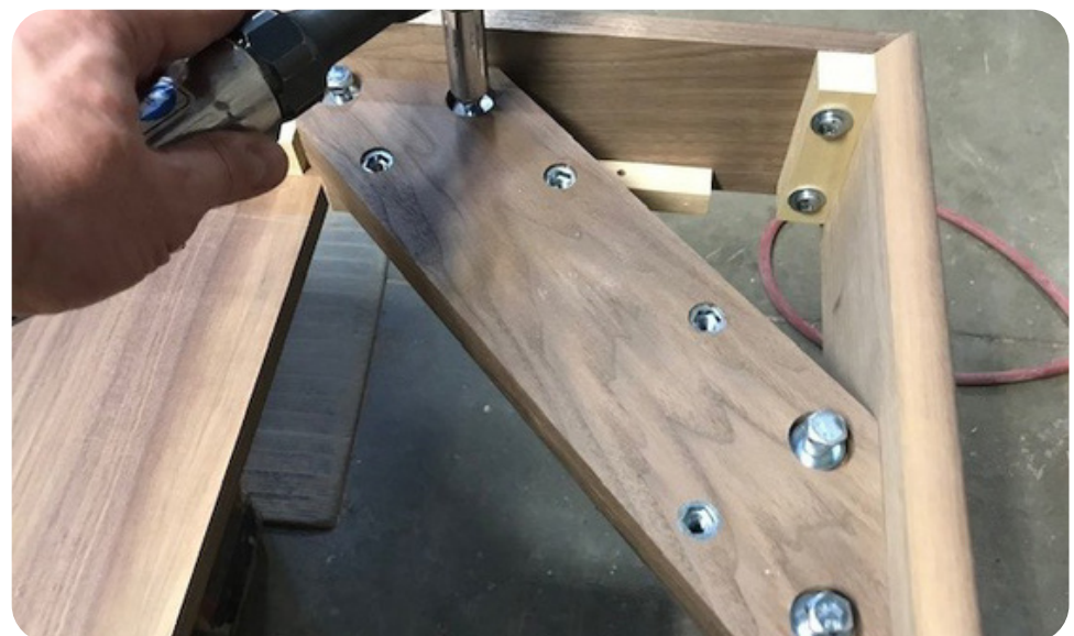
12 With help, turn upside down the assembled structure and fix the angle crossmembers with 3/8"-16 x 1 3/4" hexagonal; bolts and 13/32" flat washers.
