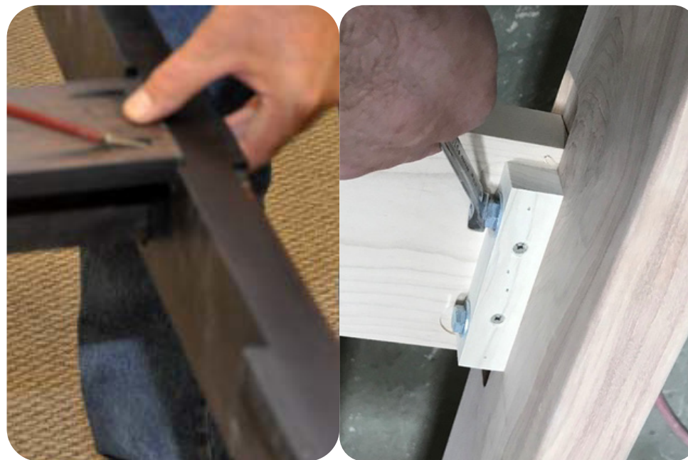
12 Screw the "T" shaped crossmembers with #8 1 1/4" wood screws and with 3/8"-16 x 1 3/4" hexagonal bolts and 7/16" flat washers fix the net crossmember
