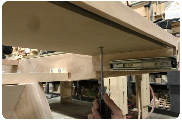
16 Repeat operations 10 and 11 for the second short apron or, for a product with a drawer, fix the drawer's box to the crossmember using 1/4"-20 x 1/2" machine screws and machine screws 1/4"-20 x 1/2" (round head). to the apron.
