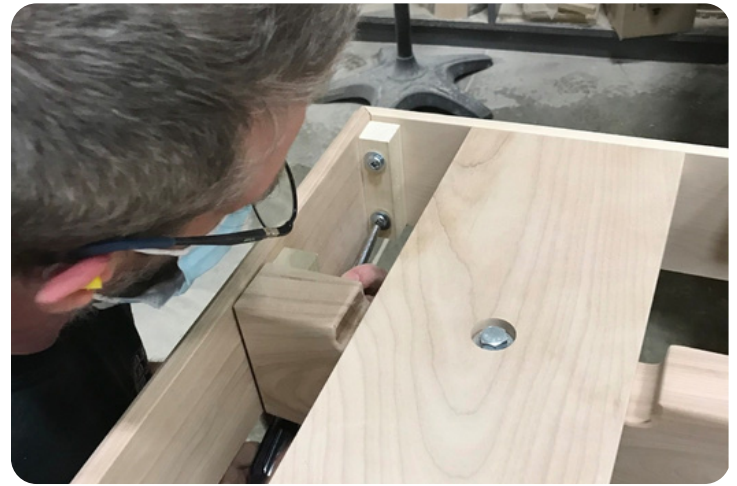
14 Fix the first short apron's corners to the long aprons with 1/4"-20 x 1 1/2" machines screws and 5/16" flat washers
