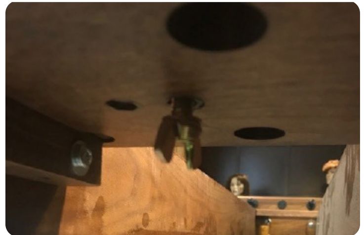
18 Loosely screw the 3/8"-16 x 1 1/2" winged nut underneath the net crossmember. This nut will allow you to tighten the net or completely remove the chrome poles when using your table as a dining table.
