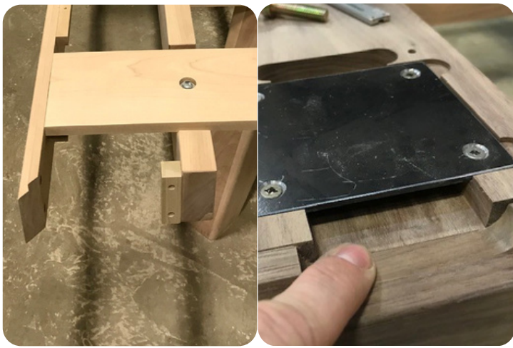
13 Fix both long aprons to the crossmembers using 1/4"-20 x 1 1/2" machines screws and 5/16" flat washers. TO FACILITATE THE INSTALLATION OF THE CHROME POLES (OPERATION 13) BE SURE THAT THE POINTED SURFACES ARE LEVELED.
