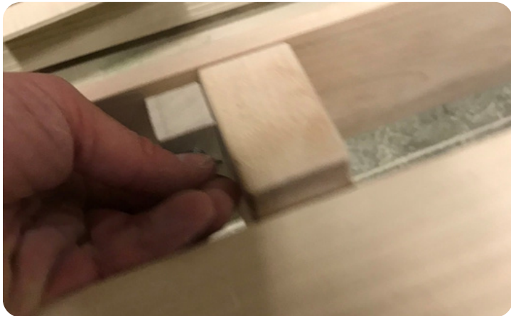
15 Fix this same short apron to the long base frames with 1/4"-20 x 1 1/2" machines screws and 5/16" flat washers
