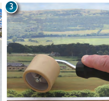
3 Roll a wallpaper seam roller over the edges to prevent them from curling. Clean its surface as you go with a damp cloth, otherwise it will spread streaks of adhesive over the backscene.
