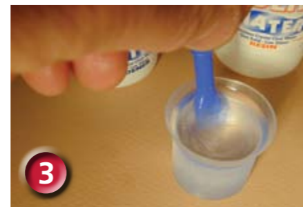
3 Mix the two together with the spatula wiping the sides of the container. Thorough mixing of the right proportions, two parts resin to one part hardener is critical! Adding more hardener will not speed up the setting and will stop the Solid Water hardening fully. The picture shows streaking meaning the resin and hardener and not full mixed yet
