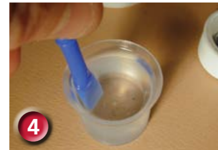
4 You can tell it's fully mixed now because it has gone clear with no streaking
