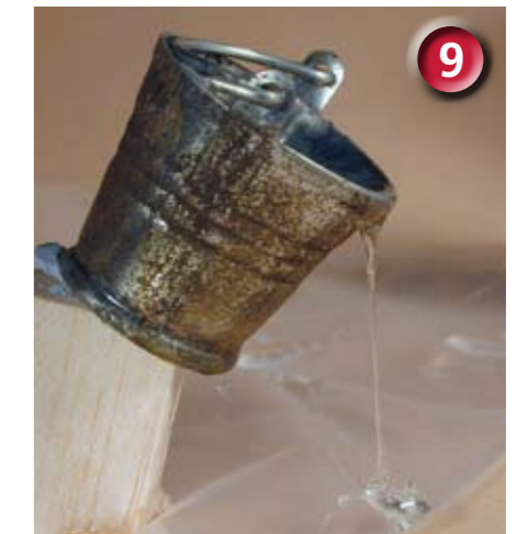
9 A heat gun or hot air dryer was useful to add fluidity to the resin and speed up both the flow and the hardening cure. Some practise here got it right first time. Leave the bucket overnight to cure
