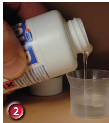
2 Use the pot to pour precisely 10ml into the mixing pot. Graduations are on the mixing pot. Add half volume of the Solid Water hardener direct from the hardener bottle
