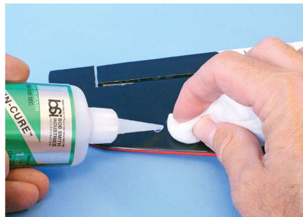
EPO foam isn't a problem for most cyanos but painted surfaces will inhibit adhesion.
