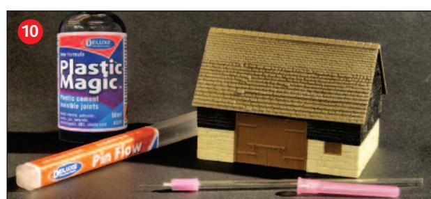
1. Drawing Plastic Magic adhesive into the Pin Flow by simply inverting the open end of the tube.
