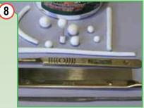
Create and Shape is one of the few one part drying materials that can be shaped in the fingers to create spheres, cylinders and other shapes without making a mess on your hands.
