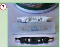
Create and Shape can replicate quite complex shapes such as this bogie frame using a mould made from silicone bath caulk. Anthracite coal will give an excellent, small scale rock strata effect. Neat washing up liquid is a great release agent.
