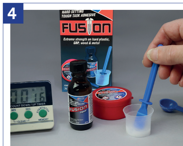
4 The mixture is stirred to wet out all the Fusion powder, which then slowly starts to dissolve into the liquid and catalyse the whole mixture.
