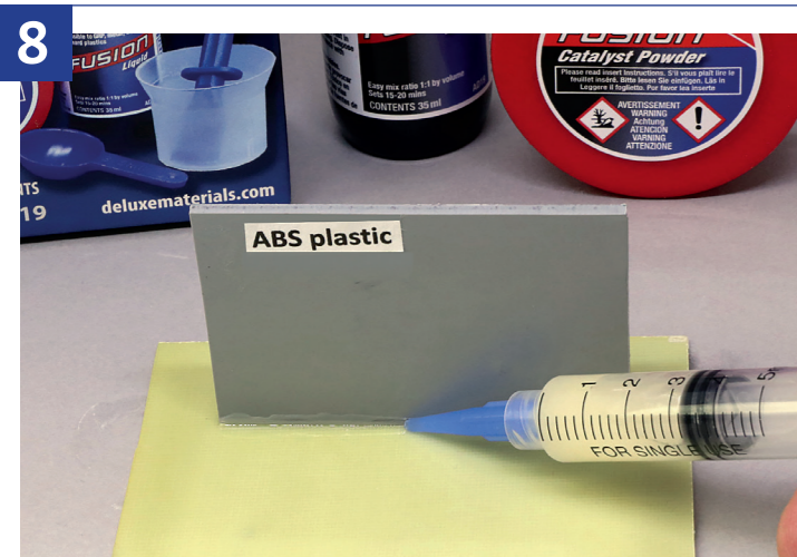
It can be applied to joints neatly using a syringe.
