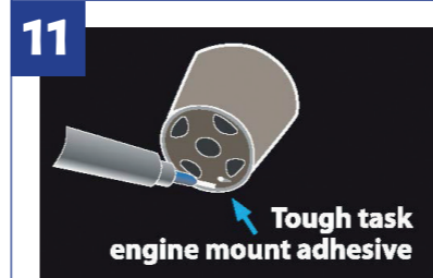
Fusion to the rescue for a critical high stress engine mount bonded into a polyester GRP fuselage.
