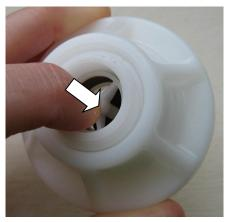
With the valve held open, submerge it in warm water with a tiny amount of washing up liquid mixed in. Move the valve backwards and forwards for a few seconds so that water is forced through the valve, removing dirt and debris. After this, flush the valve through with fresh water for one final clean.
