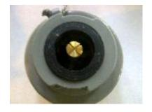
Using a pair of circlip pliers, remove the large gold coloured circlip from the body of the valve. Slide the complete spindle/diaphragm assembly up and out from inside the valve body.
