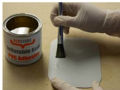
Applying the 2-part mixed adhesive to the back of the repair patch
