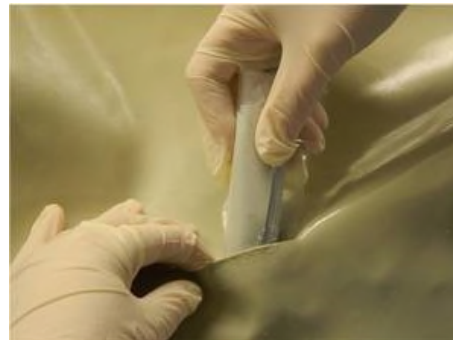
Insert the rolled-up, polythene covered, repair patch into the tube through the tear or cut in the tube.
