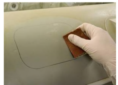
Hypalon ONLY - Abrading the repair area and back of the Hypalon fabric repair patch
