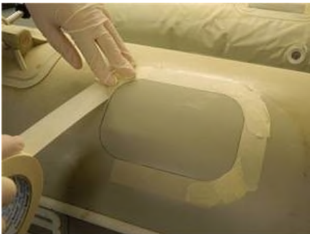
The repair area on tube being masked-up
