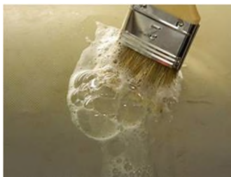
Bubbles identifying leak
