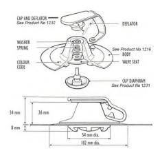
The A4 valve has been superseded by newer Leafield models that are lower in profile and easier to maintain, e.g. easier access to the rear of the valve to replace the diaphragm. However, the A4 remains a high-quality inflatable boat inflate/deflate valve that has stood the test of time.
